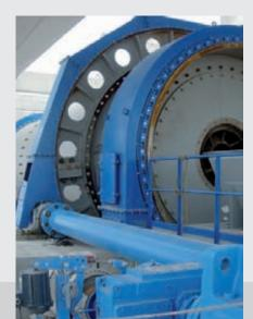
Depending on the fresh feed humidity, the cement mill can be equipped with a pre-drying chamber.
