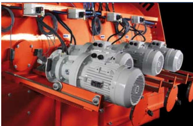
Option: agitator quick change system
