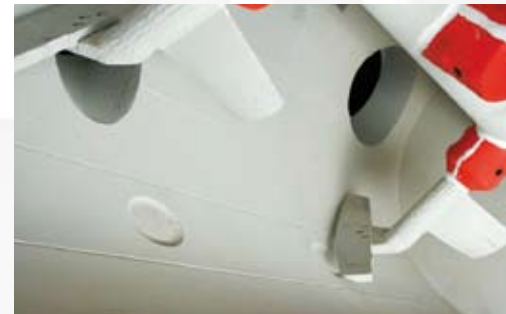
Picture shows mixing tools
