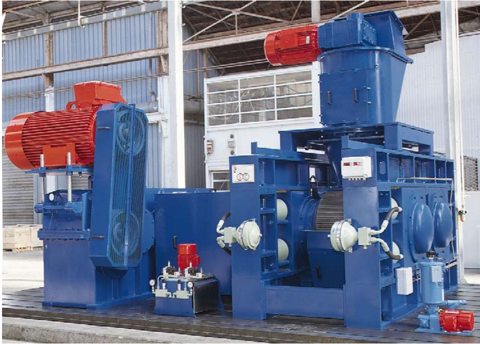
Figure 3. Compactor type HP1/800/400 - (Rolls diameter : 800 mm - Rolls width : 400 mm - Flakes capacity : 40 T/h).
