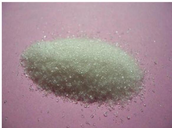
The total absorbency and swelling capacity are controlled by the type and degree of cross-linking to the polymer. Low density cross-linked **SAP** generally has a higher absorbent capacity and swells to a larger degree. These types of **SAP** also have a softer and more cohesive gel formation. High cross-link density polymers exhibit lower absorbent capacity and swell. The gel strength is firmer and can maintain particle shape even under modest pressure.
