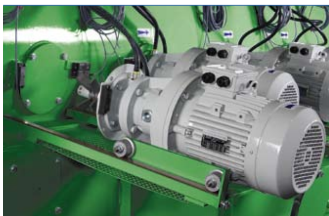
Option: agitator quick change system
